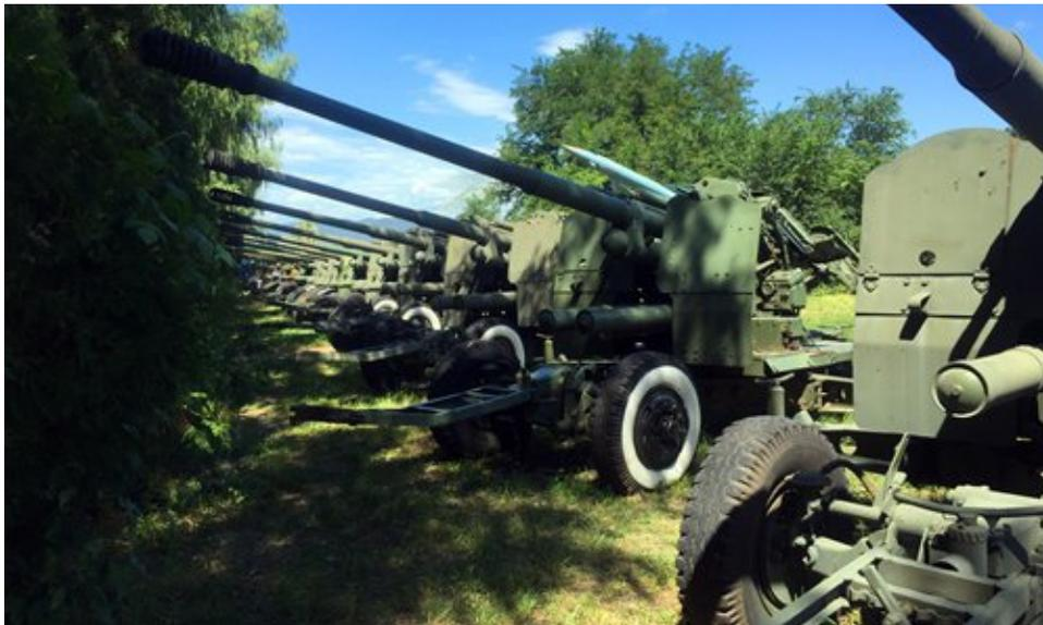
**A line of 59-type 100 mm calibre anti-aircraft artillery, which could fire 15 rounds a minute, with a range of 21 kilometers. Photo: Courtesy of Brian Salter**
